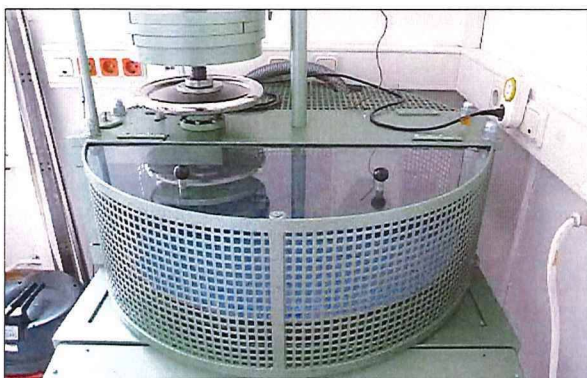
Fig. 1: Castor chair device for the determination of the resistance against soft chair rolls according to EN 425:2002
